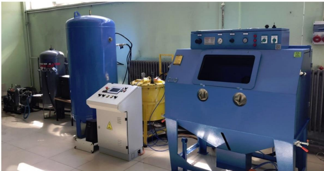
Figure 1. Solid particle erosion test system developed, a) Schematic of test system, b) Actual photo of test system
